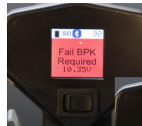
BPK-Probe test result when motor hooked up to VFD
