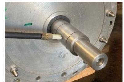
Testing shaft voltage with BPK-Probe
