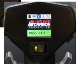
Test result when a BPK is engaged
