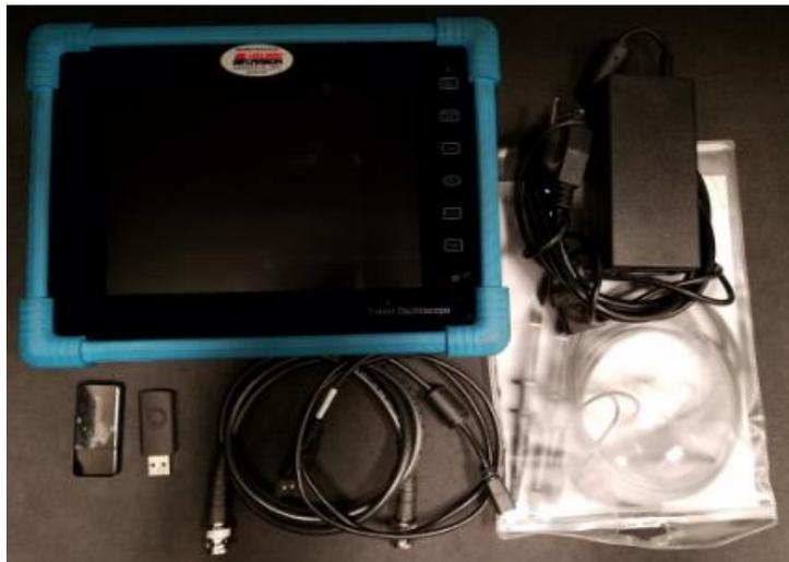
**Note:** The Tablet Oscilloscope is shipped partially charged. If the scope will not initially power up or if a recharge is needed, connect the Charger/Power Cable to a 115vac/15amp, 60Hz source. Connect the Charge Cable from the charger to the oscilloscope. For quick reference a battery status indicator is displayed in the lower right corner of the screen.
