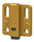
The BPK-IM5 Bearing Protector Kit is mounted using two 6-32 (included) or 3.5 mm screws (not included). The holder should be mounted 0.090" to 0.125" (2.4 mm to 3.2 mm) from the shaft.
