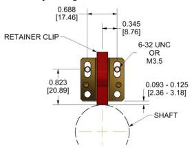
2. **Attach** holder to unit using two 6-32 or M3.5 screws.
