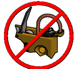
INCORRECT TERMINAL INSTALLATION
