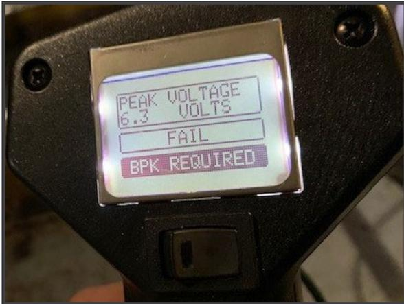
The initial BPK-Probe™ measurement displayed a FAILED, 6.3 volts on the compressor motor shaft
