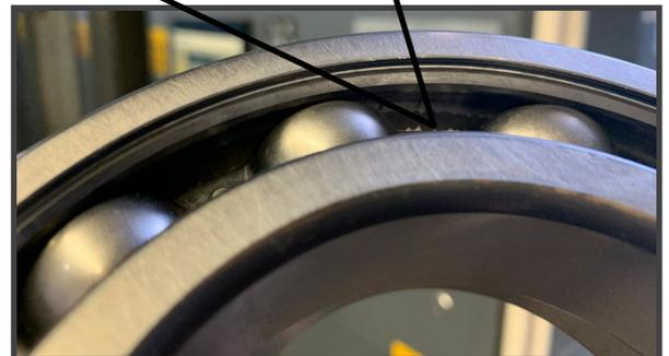
Actual damaged bearing from 243HP Siemens Motor
