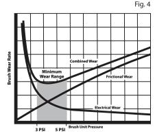
Increase in brush friction will result in the removal of the Commutator film and cause rapid brush wear. Light
