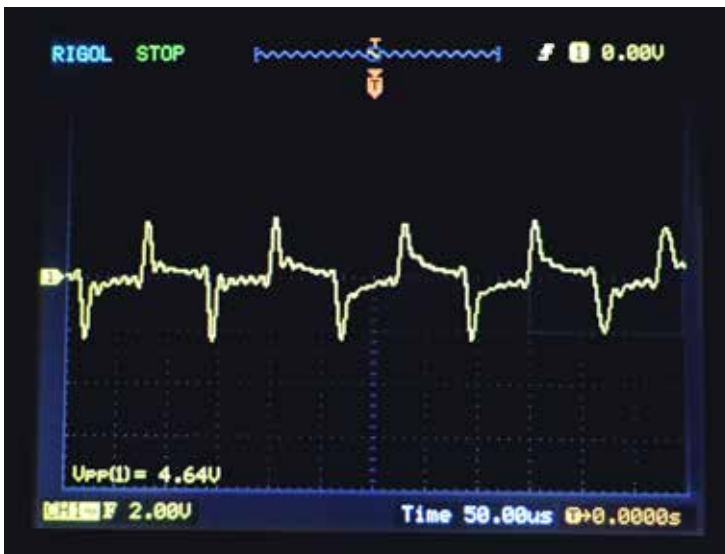
Shaft Voltage with Fiber Ring
