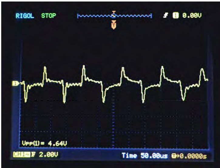
Shaft Voltage with Fiber Ring
