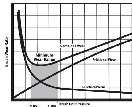
Increase in brush friction will result in the removal of the Commutator film and cause rapid brush wear. Light
